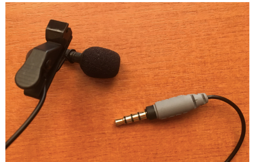
Close-up of a lavalier microphone used to record higher quality audio. The three black rings on the 3.5mm jack indicate this only works with smartphones.
